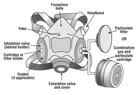
The basic parts of a typical half-facepiece respirator are shown. Two common options are illustrated on the right. Both sides of the respirator would take the same type of filter or cartridge.
